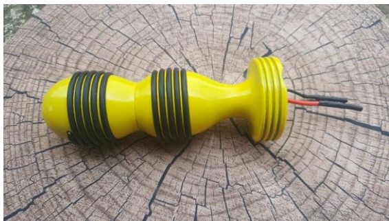
Figure 5 - Conductive rubber on one of my home made insertable electrodes
