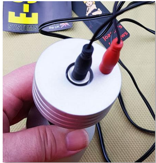
Figure 14 - Two plugs from the same cable/channel plugged into a bipolar electrode
